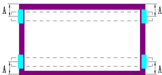
Figure H Use 4 clamps on the short side. Mounting rails run perpendicular to the short side frame. (clamp length \geq 50\text{mm} )
